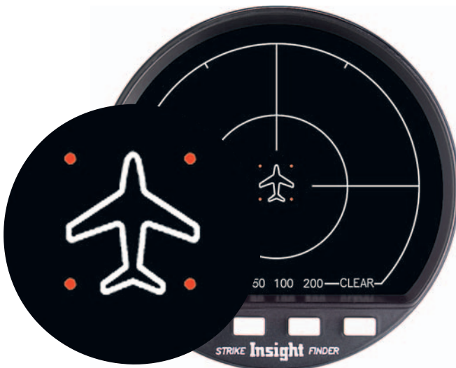
Figure 5. Display Showing Automatic Test Status Annunciator
