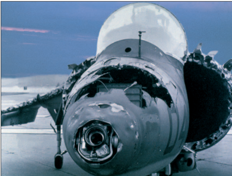
Figure 39. Aircraft Damaged by Hail
