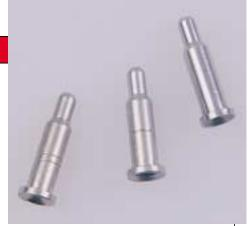
Lycoming nozzle inserts are identified by notches around the circumference of the insert. All normally aspirated engines use the single-notch insert (also used by some turbo-charged nozzles). Two-notched inserts and stepped-tube inserts (not shown) are only used on turbo-charged nozzles.
