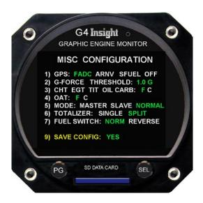
Hold PG knob in on bootup until first screen. Let go and turn PG knob to MISC CONFIGURATION screen.
