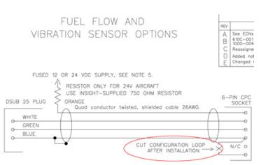
For twin engine installs with a vibration sensor on each engine:
