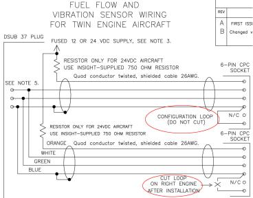
NOTE: If using 2 G3's or 2 G4 Singles cut loop on both vibration cables.
