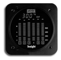
**12. GEM shows:** An increase or decrease in EGT for all cylinders, especially after engine maintenance.
