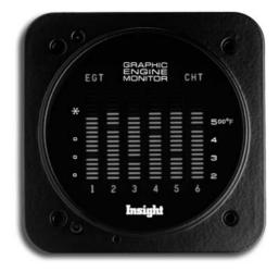
**3. GEM shows:** high CHT readings on one side of the engine (cylinders 1, 3 and 5, or 2, 4 and 6).
