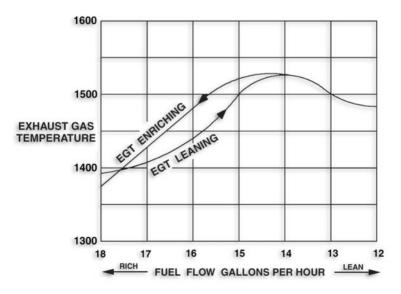
Figure 4. EGT/Fuel Flow for Turbos
