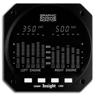
**10. GEMINI shows:** Left engine normal, right engine has a slight drop in EGT and rising CHT indications in one or more cylinders p o s s i b l y accompanied by engine roughness.
