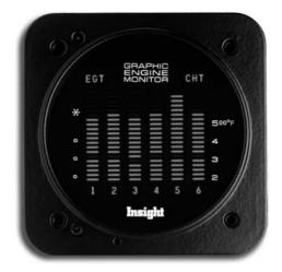
**1. GEM shows:** a gradual or sudden rise in EGT of one cylinder. When temperatures are 50°F above normal the display will blink to warn you of the rise in temperature.
