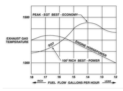
Figure 1 EGT/Fuel Flow Curve
