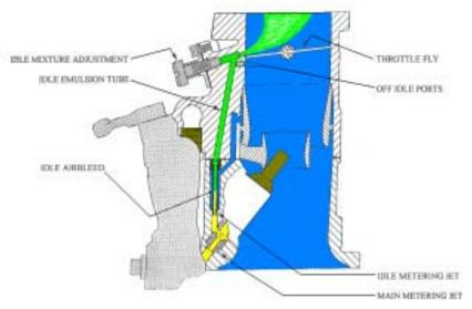
FIGURE 1. TYPICAL IDUNG SYSTEM IN A FLOAT CARBURITOR.
