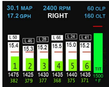
2- Turn SEL to right for right engine Tap SEL to clear lean boxes
