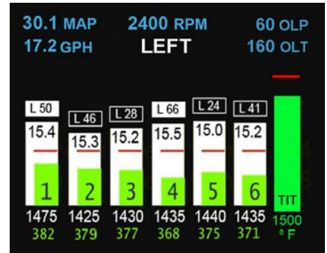
3- Turn SEL to left for left engine Tap SEL to clear lean boxes
