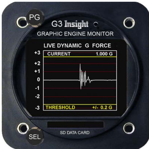
Dynamic G-Force screen SEL knob can be used to adjust screen graph size
